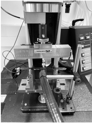
Fig. 5. Three-point beam test setup - beam and supports.
